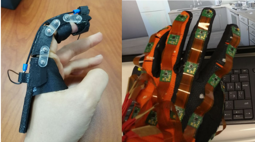
Fig. 2. Prototype with conductive cord and arm (at the left). and flexible PCB prototype with the ability to host IMU sensors (at the right)
